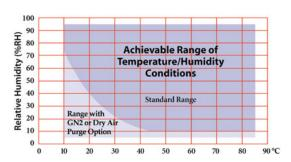
NOTE: Ability to reach RH extremes may be limited by the humidity sensor accuracy. Low Dew Point conditions can only be achieved when starting with a clean, dry chamber.
